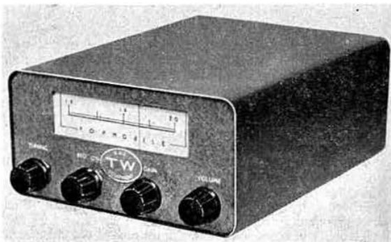
The Withers "Topmobile" transistor receiver for 1.8-2 Mc/s. A model covering 144-146 Mc/s is also available. (Photo by courtesy of Withers Electronics)
