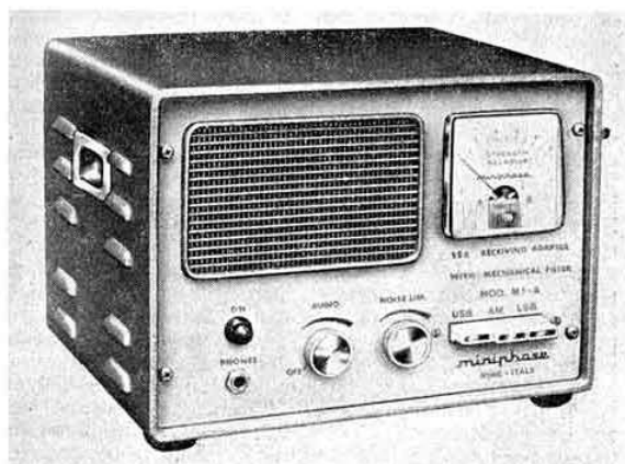
A front view of the Miniphase s.s.b. receiving adapter showing the positions of the various controls. The mode of reception is selected by the press button switches at the bottom right.
